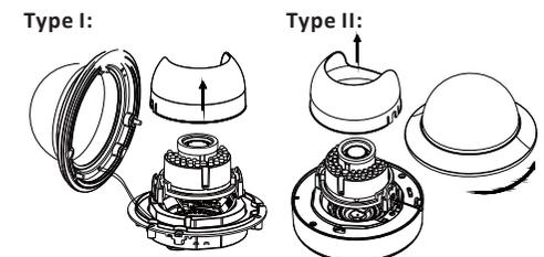
Figure 2-2 Remove the Bubble
