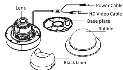
Figure 1-2 Overview of Type II Dome Camera
