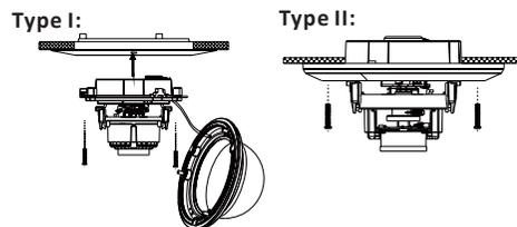
Figure 2-6 Fix the Camera to the Mount
