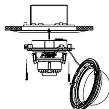
Figure 2-8 Fix the Camera to the Gang Box
