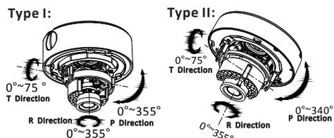
Figure 2-4 3-axis Adjustment
