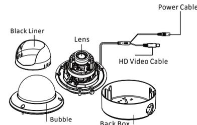
Figure 1-1 Overview of Type I Dome Camera
