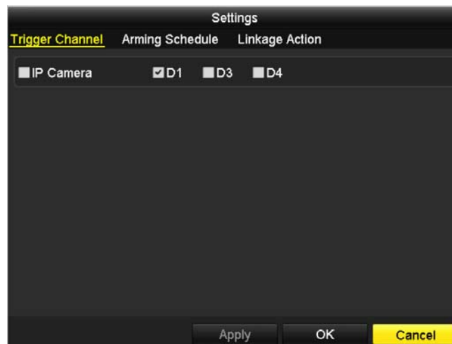
Figure 5. 13 Motion Detection Handling
