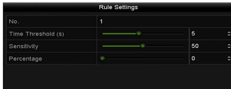
Figure 9. 6 Set Intrusion Crossing Detection Rules
