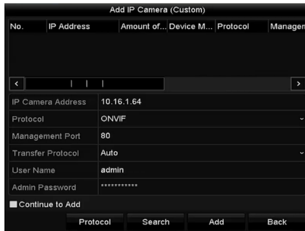
Figure 2. 28 Custom Adding IP Camera Interface
