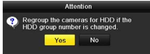
Figure 12. 14 Confirm HDD Group Settings
