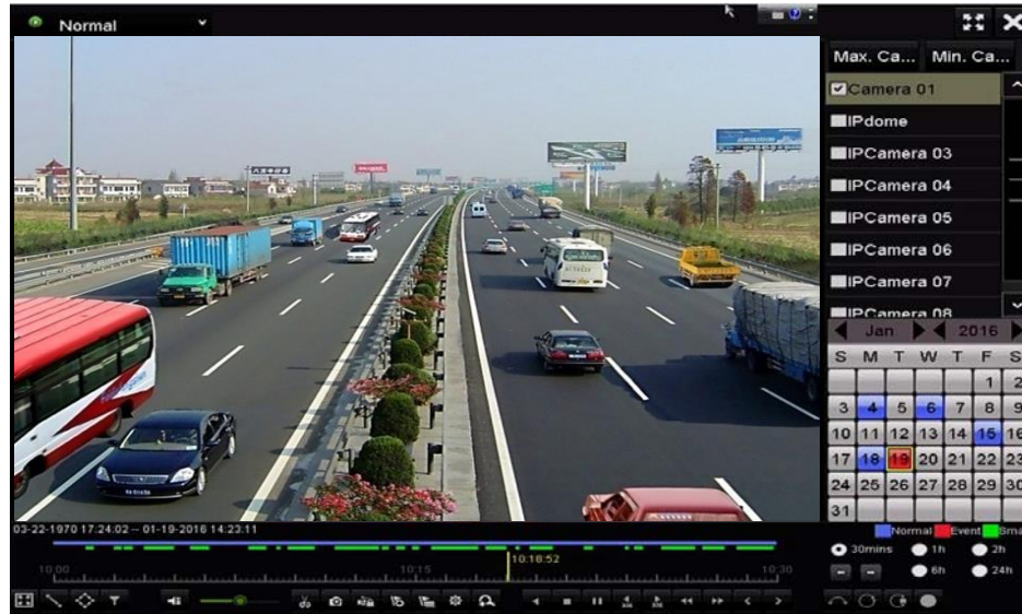
Figure 6.12 Interface of Playback by Time
