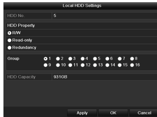
Figure 12. 13 Local HDD Settings Interface
