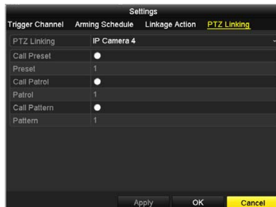
Figure 8.6 Set PTZ Linking of Alarm Input
