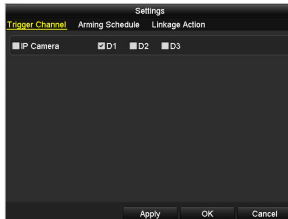
Figure 8. 1 Set Trigger Camera of Motion Detection
