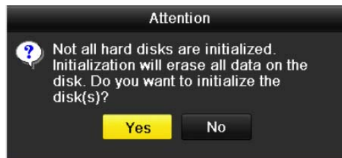
Figure 12. 1 Message Box of Uninitialized HDD
