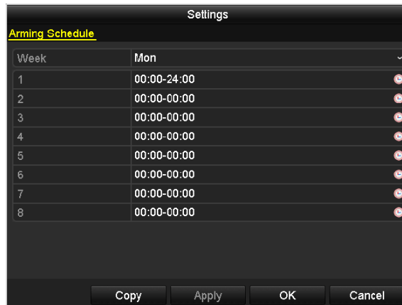
Figure 8. 16 Set Arming Schedule of Alarm Output
