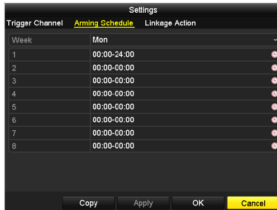
Figure 8. 2 Set Arming Schedule of Motion Detection
