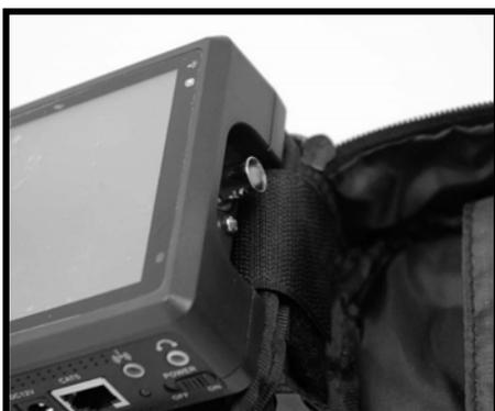
Pull the strap through and stick it tightly across the case joint to the Velcro on the opposite side.
