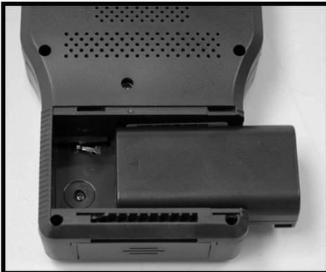
When installing the battery, please ensure that it is orientated correctly as shown in the figure.
