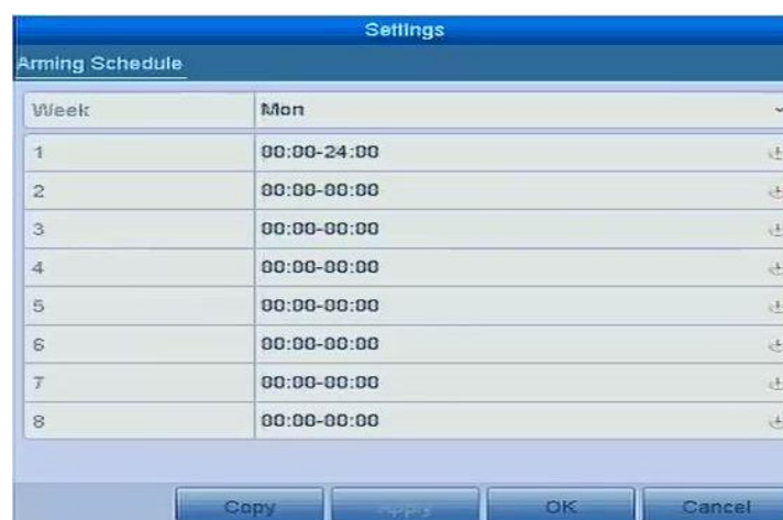
Figure 8.15 Set Arming Schedule of Alarm Output
