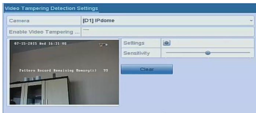
Figure 8.9 Video Tampering Setup Interface
