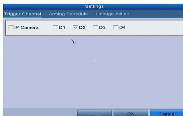
Figure 5. 17 Set Trigger Camera of VCA Alarm
