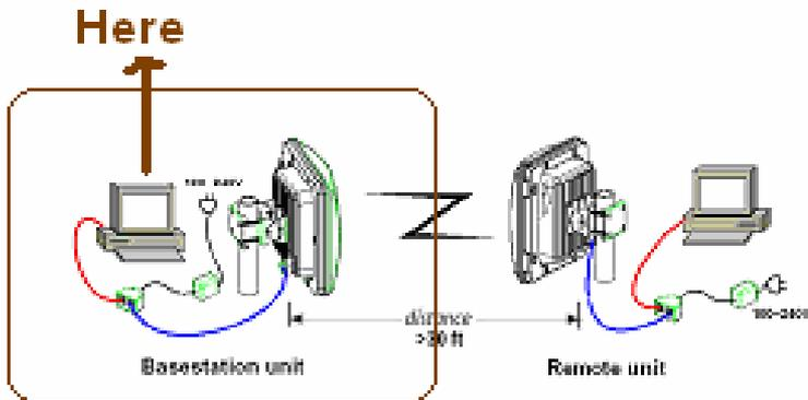
Step 3: To test the data rate when pressing the test.
