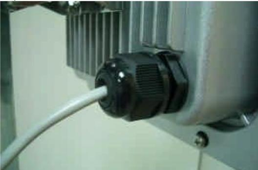
Step 2: Connect the Ethernet cable to PoE Splitter set
