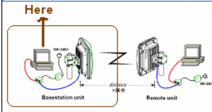
Step 4: Data rate will be lower if the radiative angle of Antenna is wrong.
